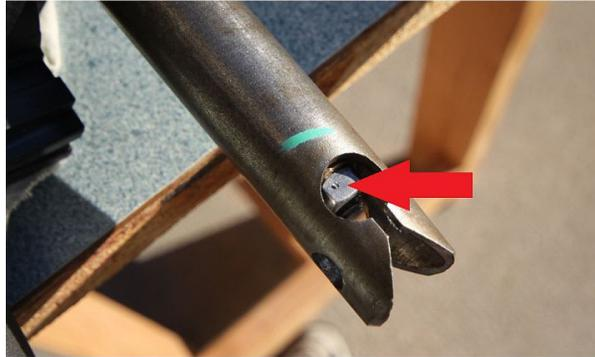
8. Install motor – First smooth out the roll pin with your grinder. This will make it easier to hammer in or you could use the other side. Put the motor in place and hammer the roll pin in gently. The roll pin will be shorter but it fits in so tight it won't move. You could use a ¼ bolt, but the motor tends to twist more than normal. The roll pin is slightly oversized, thus a much tighter fit. If the roll pin is too damaged, a ¼ sized one can be bought at a home supply store.
