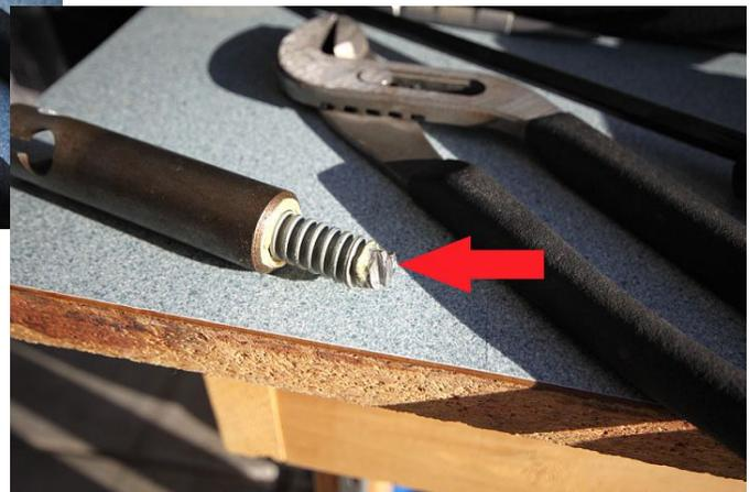
Cut a notch to help unscrew the shaft from the tube nut
